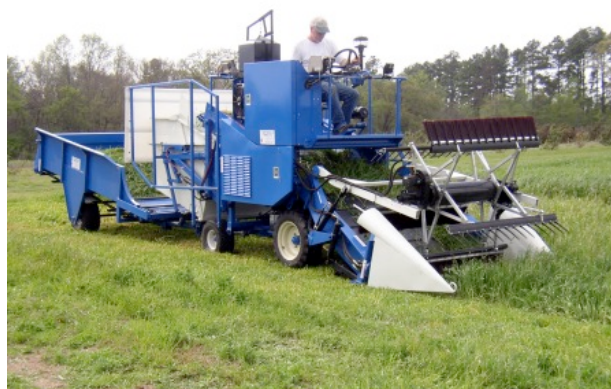
Fig. 1. Swift Machine forage plot harvester with collection/dump trailer.
