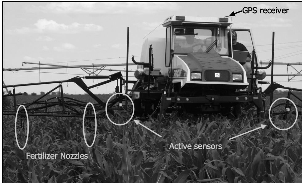
Fig. 1. Pictured above is the high clearance N applicator configured with active crop canopy sensors along with fertilizer delivery system, consisting of two-drop nozzles/valves placed at alternating rows of corn. Depending on the configuration of valves turned on/off, system can deliver a multiple of 4 rates of liquid N fertilizer on-the-go as directed by the controller system interfaced to the active sensor.
