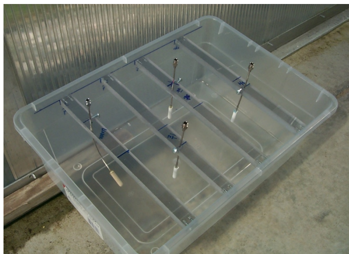
Figure 1. Container and lysimeter design for Phase I.
