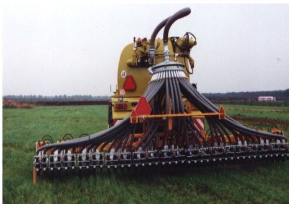
Figure 11. Inject biosolids directly into sod.
