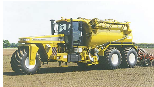
Figure 8. High flotation applicator with positive displacement pump.
