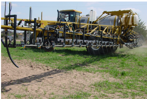
Figure 6. TerraGator with GreenSeeker mounted in combination with the standard system.
