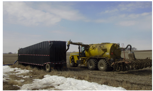
Figure 9. Load 4500 gal in 3.5 minutes from a field side reservoir without leaving the cab.
