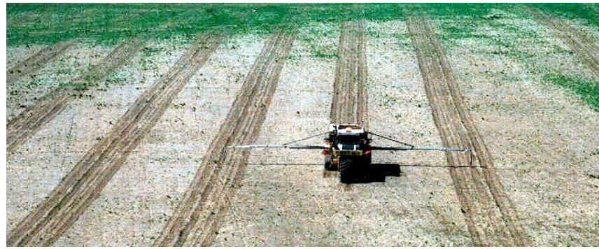
Figure 1. TerraGator equipped with Auto-Guide applying fertilizer.
