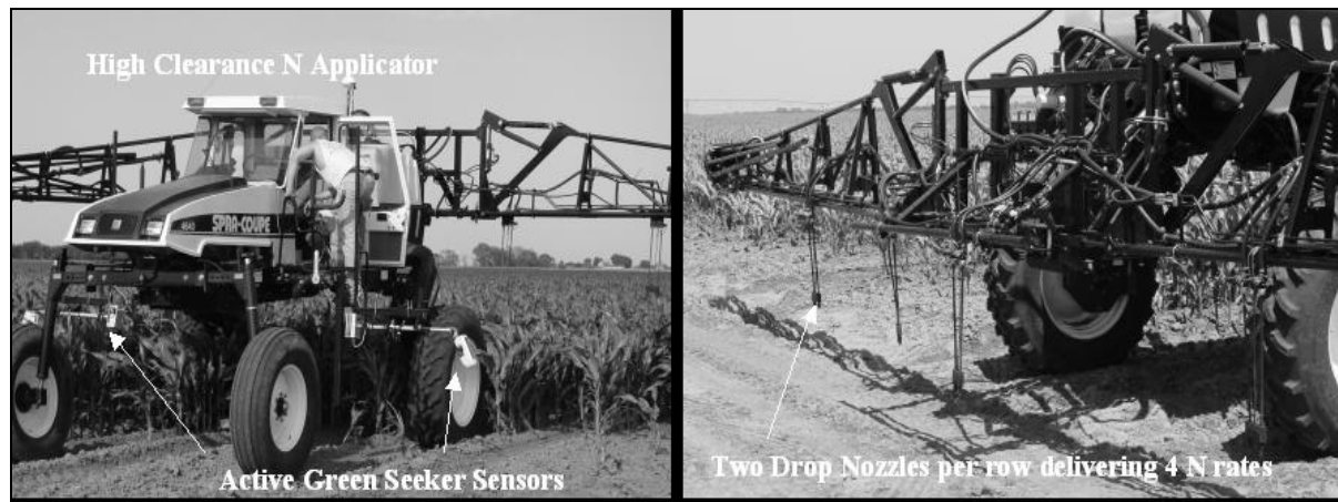
Figure 2. Pictured upper left is the high clearance N applicator illustrating key components, including the active GreenSeeker® crop canopy sensor mounted on front. Both the red and green versions of the active sensor manufactured by Ntech Industries, Inc. ( http://www.ntechindustries.com/ ) were tested and evaluated. Shown in the upper right image is the liquid N fertilizer delivery system, consisting of two-drop nozzles/valves placed at alternating rows of corn. Depending on the configuration of valves turned on/off, the system can deliver a multiple of four (i.e., (0, 45, 90, 135 kg N/ha) rates of liquid N fertilizer on-the-go as directed by the controller system interfaced to the active sensor or with a prescription map.
