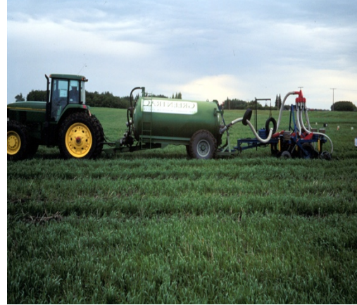
Figure 1. Low disturbance disc systems for injecting liquid manure.
