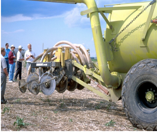
Figure 1. Low disturbance disc systems for injecting liquid manure.
