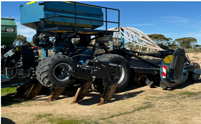
The spader used for ameliorating the soil. The front view shows the clay delving tynes that lift the clay to the surface, followed by the mixing action of the spader and then the seeder to place the seed and fertiliser, with the press wheels to firm the seedbed and assist with germination.
